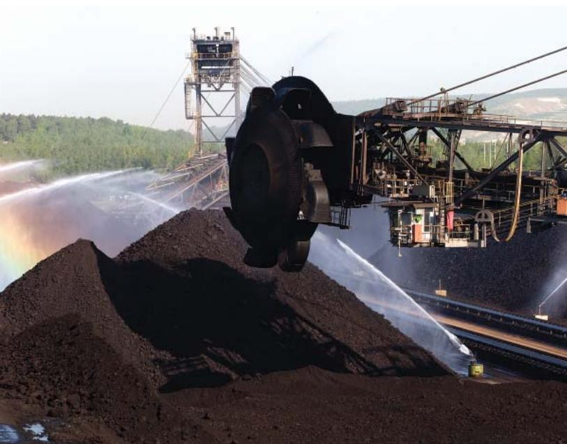
Dust mitigation measures at a coal handling facility. (Photo: RWE Mining)
