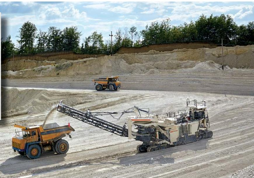
The 2500 SM from Wirtgen mining limestone in Ukraine. Inset: A satisfied customer! A view inside the 2500 SM cab. (Photos: Wirtgen)
